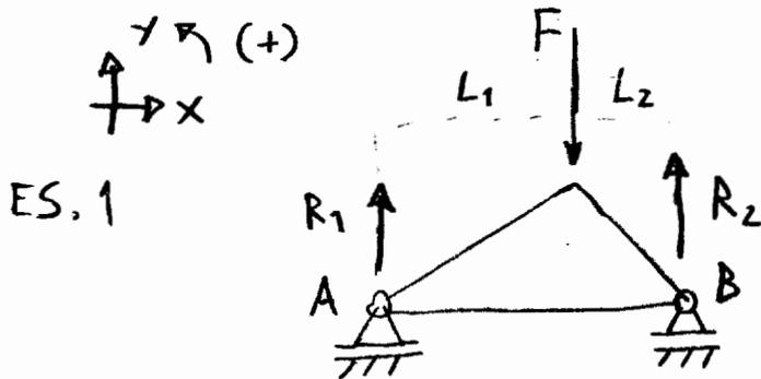
$$\begin{cases} R_1 + R_2 - F = 0 \\ 0 \times R_1 + R_2 (L_1 + L_2) - F L_1 = 0 \end{cases}$$
