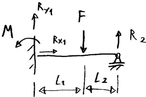
$$\begin{cases} R_{x1} = 0 \\ R_{y1} + R_2 - F = 0 \\ M - F L_1 + R_2 (L_1 + L_2) = 0 \end{cases}$$
