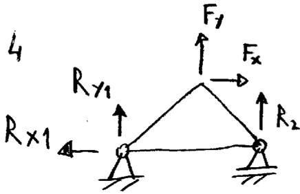
$$\begin{cases} F_x - R_{x1} = 0 \\ R_{y1} + R_2 - F_y = 0 \\ R_2(L_1 + L_2) - F_x H - F_y L_1 = 0 \end{cases}$$
